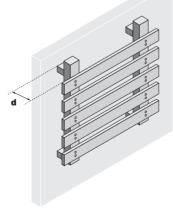
5. Installed on flat. ModWood can be installed on top of or under the frame. (ensure sub frame is adequately engineered)
